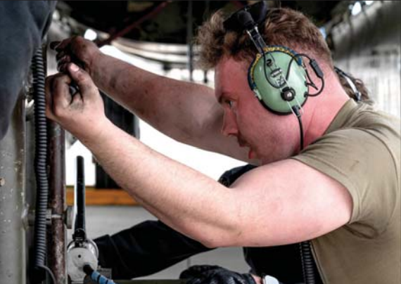
Senior Airman Zachary Cecchini, 23rd Bomber Generation Squadron crew chief, installs a tire on a U.S. Air Force B-52H Stratofortress during Red Flag 25-2 at Nellis Air Force Base, Nevada, March 12, 2025. Cecchini assisted his team with several maintenance tasks during Red Flag 25-2.
