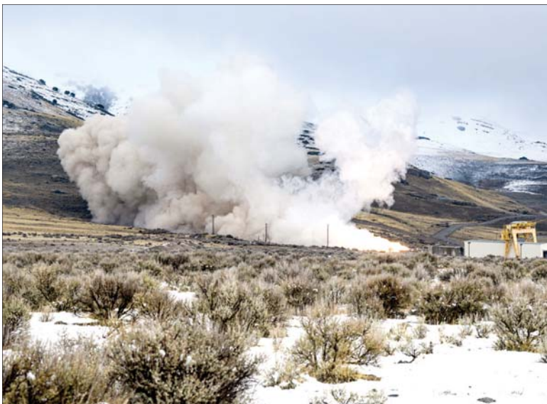
The U.S. Air Force and Northrop Grumman Corporation conduct a full-scale qualification static fire test of the Sentinel intercontinental ballistic missile (ICBM) stage-one solid rocket motor March 6, 2025, at Northrop Grumman's facility in Promontory, Utah. The Sentinel program is modernizing the land-based leg of the U.S. nuclear triad, replacing the aging Minuteman III ICBM weapon system.
