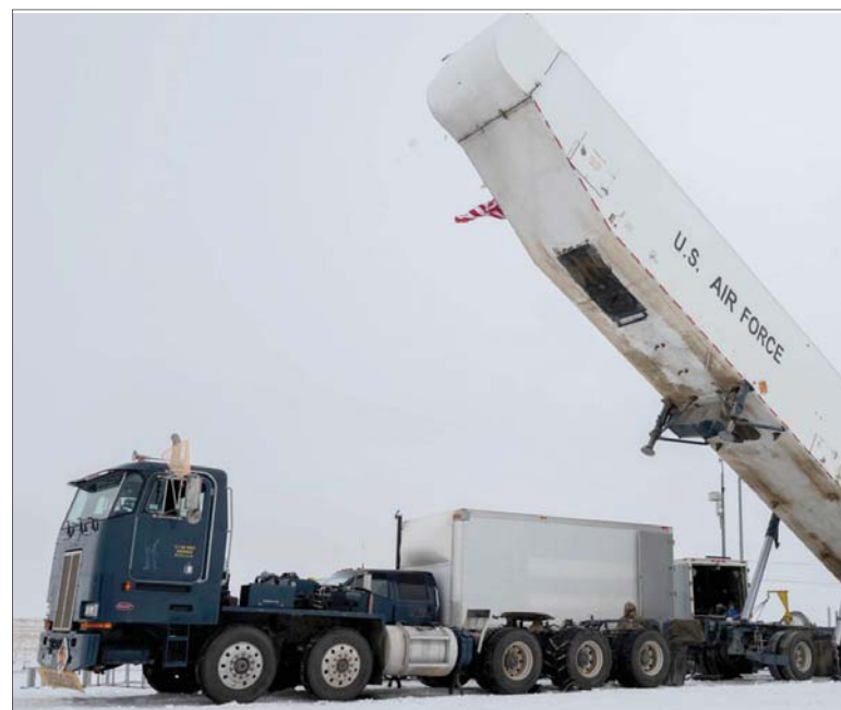
Airmen assigned to the 91st Missile Maintenance Squadron use a transporter erector to accomplish Minuteman III missile maintenance at Minot Air Force Base, North Dakota, Jan. 14, 2025. The transporter erector has been a piece of equipment used since its creation in the late 1980s and has served as a reliable and efficient way of performing missile maintenance and transport.
