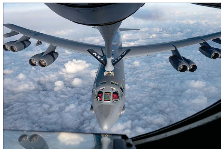
A U.S. Air Force B-52 Stratofortress from the 5th Bomb Wing, Minot Air Force Base, North Dakota, receives fuel from a KC-135 Stratotanker from the 100th Air Refueling Wing, Royal Air Force Mildenhall, England, over the North Sea, Sept. 11, 2024. Bomber task force missions are representative of the U.S.’ extended deterrent commitment to Allies and partners and enhance regional security.
