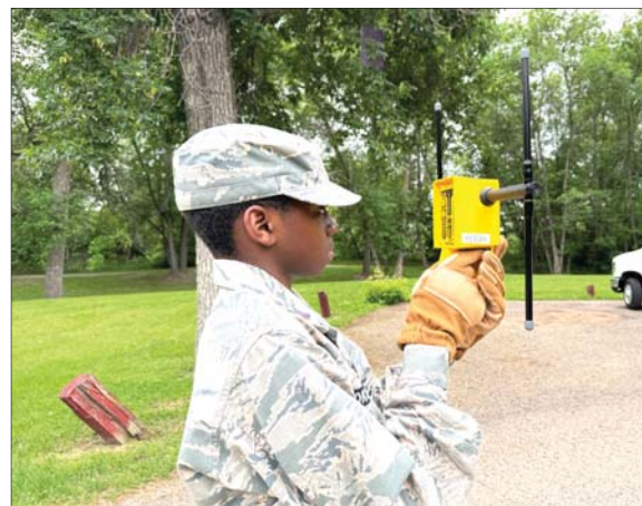
Cadet Favour Okonkwo uses a digital receiver to find a training emergency locator beacon, similar to beacons installed in all general aviation aircraft.
