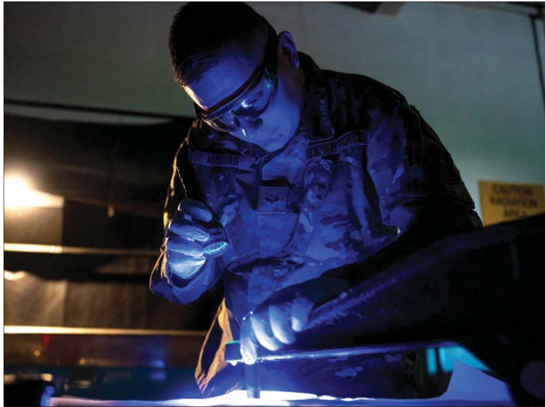
U.S. Air Force Senior Airman Jonathan Macias, 5th Maintenance Squadron non-destructive inspection (NDI) journeyman, inspects a MHU-97/E part during a magnetic particle inspection at Minot Air Force Base, North Dakota, June 6, 2024. NDI technicians use various methods to inspect metal objects to ensure they remain properly functional.
