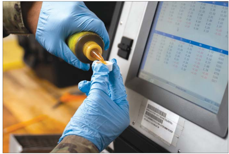
U.S. Air Force Airman 1st Class Omar Murphy, 5th Maintenance Squadron non-destructive inspection (NDI) apprentice, demonstrates an oil analysis at Minot Air Force Base, North Dakota, June 6, 2024. NDI has a variety of inspection methods, to include fluorescent penetrant, magnetic particles, x-ray, ultrasound, oil analysis and eddy current.
