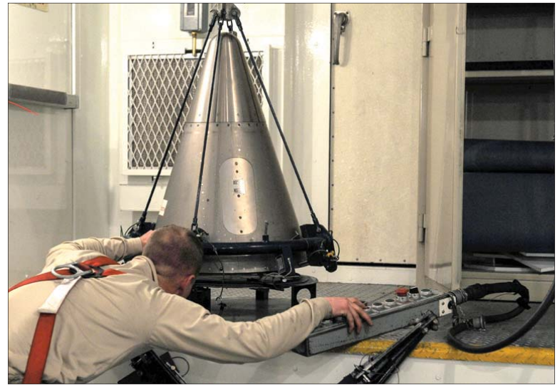
Senior Airman Andrew Parrish, 90th Missile Maintenance Squadron topside technician, prepares the forward section, of a reentry system, for secure transportation, Feb. 2, 2018, in the F. E. Warren Air Force Base missile complex. 90th MMXS Airmen transport missile components and perform maintenance across a 9,600 square mile tristate area. Missile maintenance teams perform periodic maintenance to maintain the on-alert status for launch facilities, ensuring the success of the nuclear deterrence mission.
