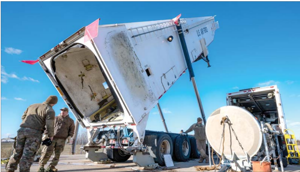
U.S. Air Force Staff Sgt. Ethan Bowman, 91st Missile Maintenance Squadron missile handling team chief, observes his team retracting a Transporter Erector during a training exercise at Minot Air Force Base, North Dakota, Nov. 16, 2023. The Transporter Erector transports, stores, removes and emplaces the Minuteman III Missile.
