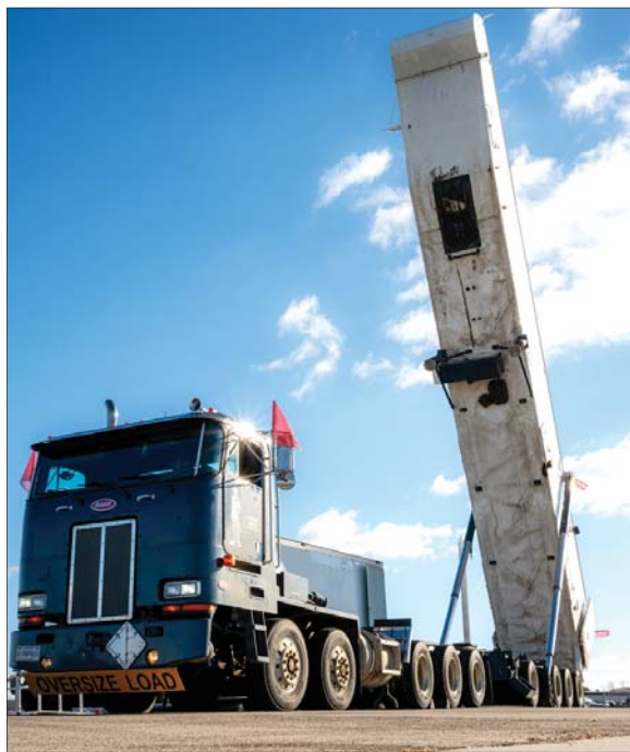
A Transporter Erector retracts during a training exercise at Minot Air Force Base, North Dakota, Nov. 16, 2023. The Transporter Erector is used to lower the Minute Man III, into one of many missile silos around Minot AFB's area of responsibility
