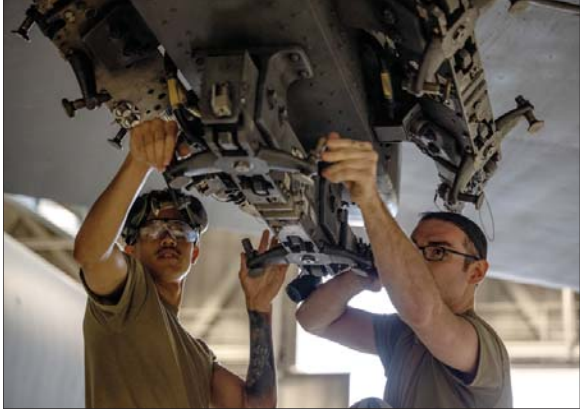
Airman 1st Class Timothy McDonald, 5th Aircraft Maintenance Squadron weapons load crew member (left), and Senior Airman Matthew McMahon, 5th Aircraft Maintenance Squadron weapons load crew member (right), load an inert precision guided munition onto a B-52H Stratofortress at Minot Air Force Base, North Dakota, Oct. 2, 2023. The Airmen competed in the 3rd Quarter Load Crew Competition evaluating their preparedness.
