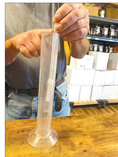
An alcohol hydrometer is used to test the alcohol content of each batch of wine
