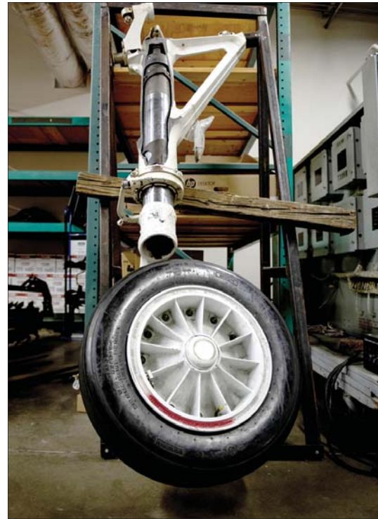
A broken B-52H Stratofortress tip landing gear used for training is displayed at the 372nd Training Squadron, Detachment 22 at Minot Air Force Base, North Dakota, Aug. 28, 2023. The training at Det. 22 is important because it offers hands-on familiarization for new Airmen without impacting flight line operations.
