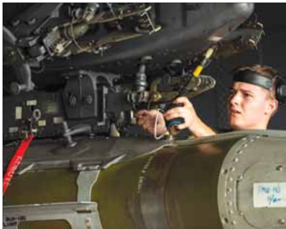
Senior Airman Cody Brittain, 5th Aircraft Maintenance Squadron load crew member, attaches an inert precision guided munition to the wing pylon of a B-52H Stratofortress at Minot Air Force Base, North Dakota, July 14, 2023. Brittain and his team competed in a quarterly weapons load competition testing readiness.
