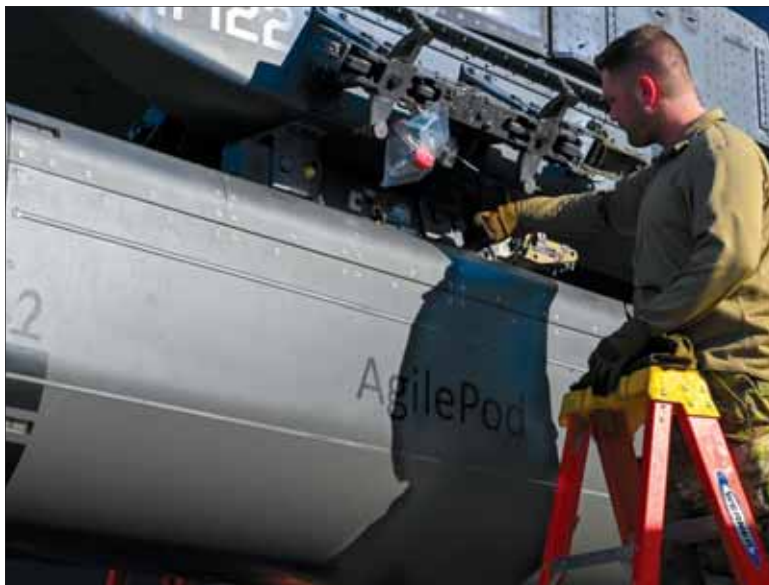
TSgt Andrew Groff, 307th Aircraft Maintenance Squadron aircraft armament technician, adjusts an AgilePod onto a B-52 Stratofortress, at Barksdale Air Force Base, Louisiana, Jan. 10, 2023. The AgilePod is a multi-function pod built to integrate advanced communications capabilities for the B-52 across all domains.
