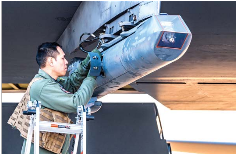
Capt. Angelico Palparan, weapon system officer assigned to the 23rd Expeditionary Bomb Squadron, inspects a B-52H Stratofortress targeting pod before takeoff at Morón Air Base, Spain, Mar. 1, 2023. Strategic bomber missions enhance the readiness and training necessary to respond to any potential crisis or challenge across the globe.
