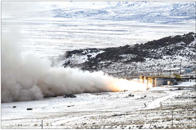
The Air Force Nuclear Weapons Center conducted its first full-scale static test fire of the LGM-35A Sentinel stage-one solid rocket motor at the Northrop Grumman test facility in Promontory, Utah, March 2, 2023. The Air Force plans to replace the fielded Minuteman III intercontinental ballistic missile with the next-generation Sentinel system currently in development. The Sentinel acquisition program represents the modernization of the land-based leg of the U.S. nuclear triad.
